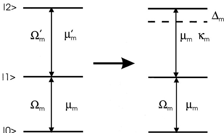
**Figure 2** Mapping of the three-level system (*left*) onto the excitonic-oscillator (quasiparticle) model (*right*).  $\Delta_m = \Omega'_m - \Omega_m$  is the anharmonicity parameter.  $\kappa_m$  represents the ratio of the two transition dipoles.
