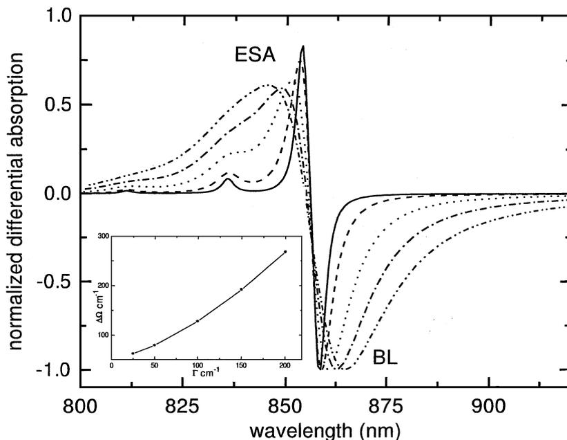
**Figure 6** Normalized pump-probe spectra of the LH2 antenna without disorder for different dephasing rates  $\Gamma$  at 4.2 K.  $\kappa = 0.9$ .  $\Gamma =$  (solid)  $25 \text{ cm}^{-1}$ , (dash)  $50 \text{ cm}^{-1}$ , (dot)  $100 \text{ cm}^{-1}$ , (dash-dot)  $150 \text{ cm}^{-1}$ , and (dash-dot-dot)  $200 \text{ cm}^{-1}$ . (Inset) Peak splitting  $\Delta\Omega$  as a function of  $\Gamma$ . For other parameters see text. ESA, Excited state absorption (73).
