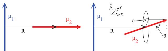
FIG. 2. Left: Sketch of the arrangement of the two transition dipole moments  $\mu_1$  and  $\mu_2$  and the connecting vector  $\mathbf{R}$  of the PBDA pair. Right: Illustration of the angle  $\theta$  and  $\phi$  when  $\mu_2$  does not point along the  $x$ -axis.
