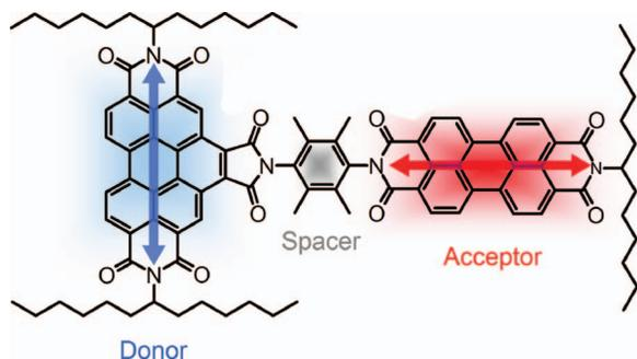
FIG. 1. Sketch of the chemical structure of an orthogonally arranged perylene bisimide donor-acceptor pair (PBDA) together with the transition dipole moments.<sup>12</sup>
